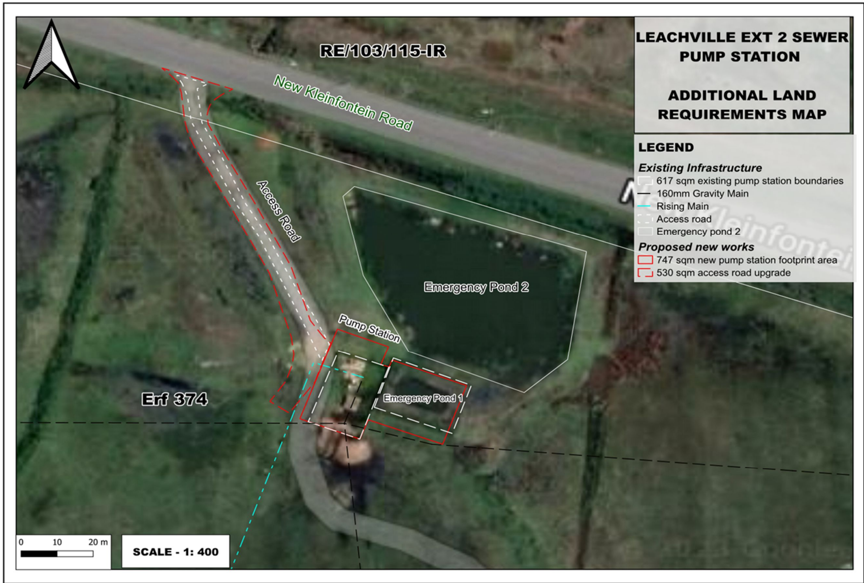
Figure 1: Map showing the existing pump station infrastructure and the proposed expansion area.
