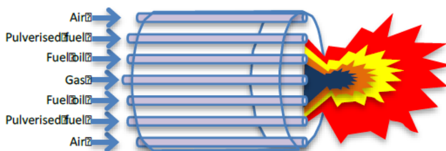
Figure 6 Simplified schematic presentation of a low NOx burner. The incoming air is controlled in such a way that flame temperature is reduced, thereby limiting the formation of NOx formation (SE Solutions (Pty) Ltd, 2013)
