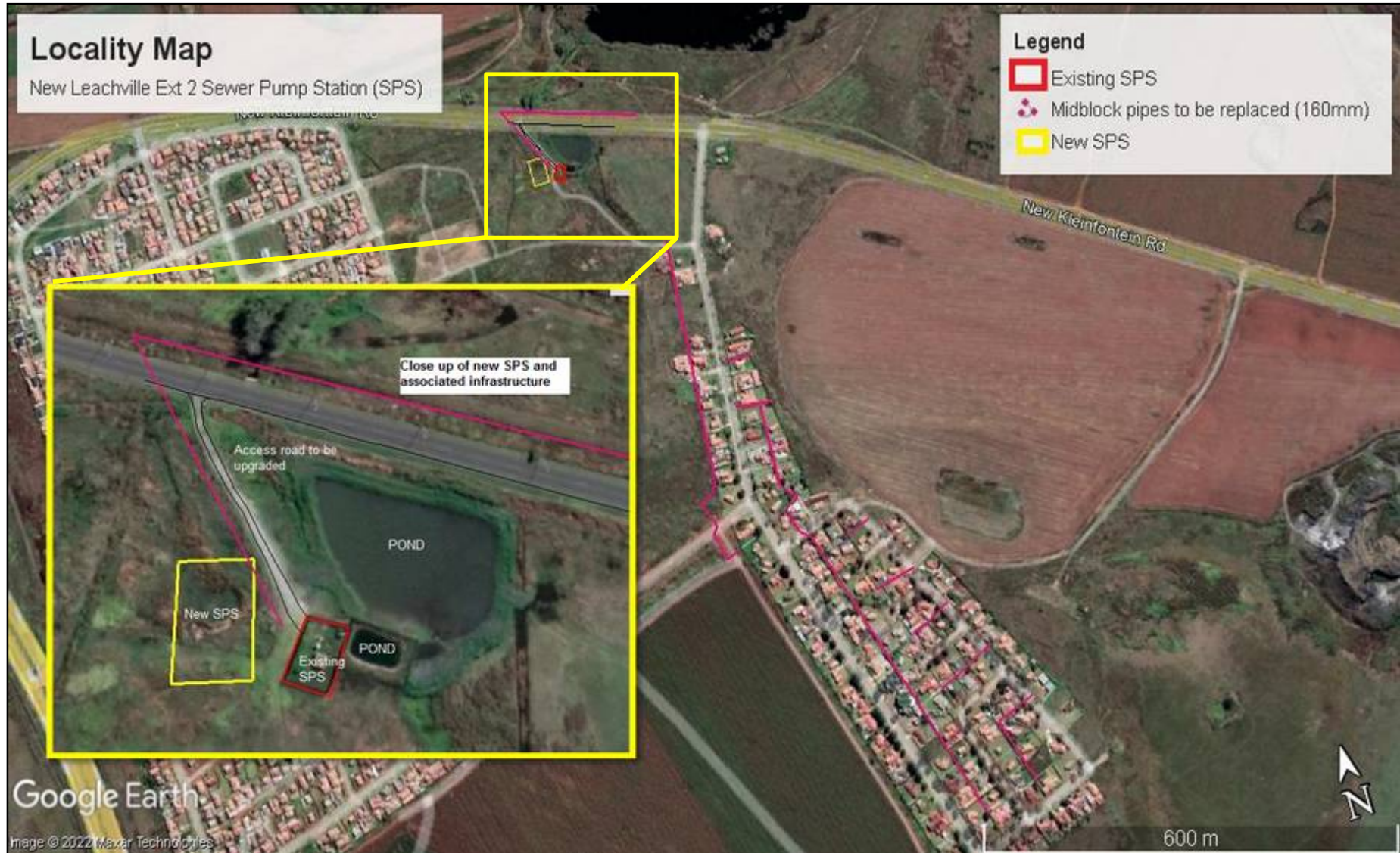
Figure 4: Google Earth Satellite Imagery showing the location of the new sewer pump station (yellow polygon), road upgrade (black) and midblock pipes to be replaced (pink line). The majority of the pipes to be replaced are located within a road reserve and an urban area.
